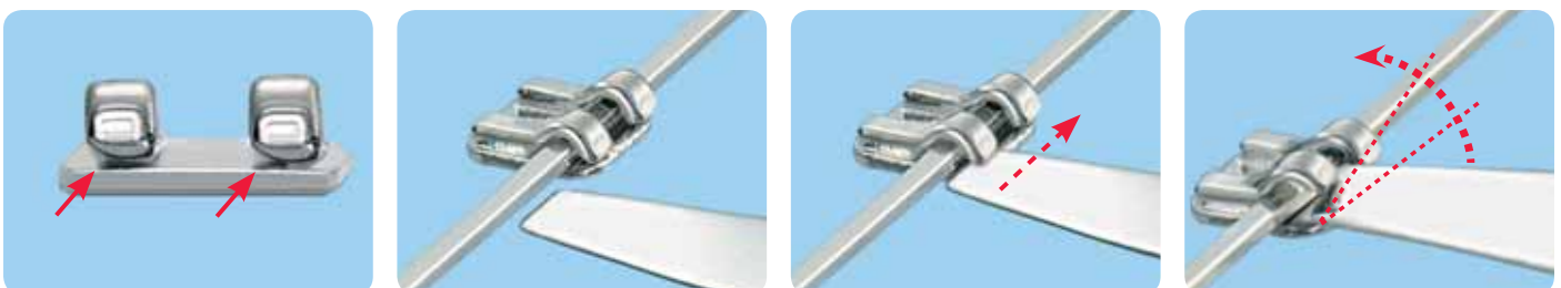
The 2D® lingual bracket is easy to open. Just slide the special explorer between clip and bracket base and open the clip by lever movement.
